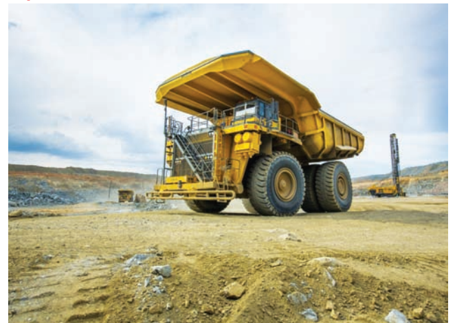
An example of a mine haul truck that will be converted to run on hydrogen. Credit: Anglo American Plc.
