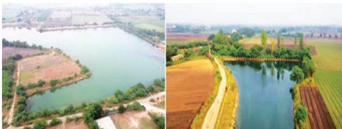
Fig. 10: Final mine closure of Solaj Limestone Mine of M/s Ambuja Cements Ltd. with water reservoir with peripheral plantations
