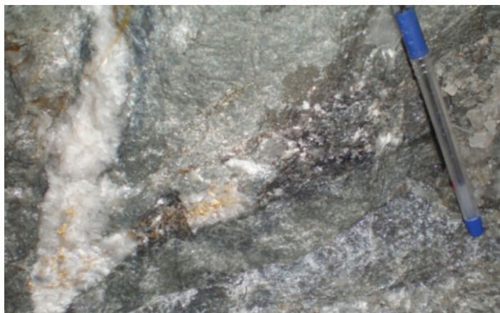
Fig. 8 Intersection of quartz vein with coarse gold in exploratory underground development drive at ATR 13.
