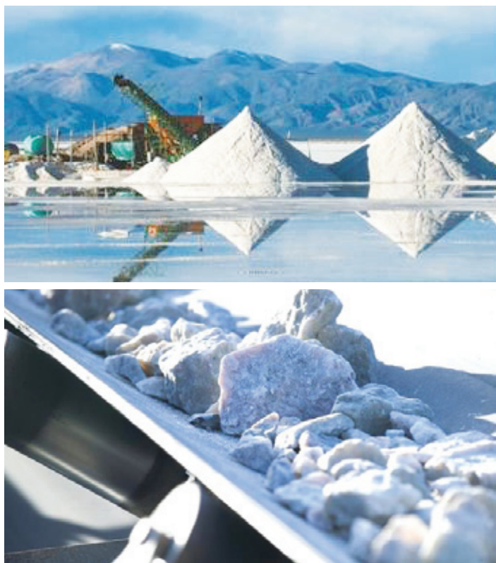
Fig.2 (L) Lithium extraction from brine: At the Salinas Grandes salt flats in Argentina, lithium is extracted on a large scale by evaporating ancient brine (image: Kramer D, 2021); Bolivia holds the world's largest lithium resources that are yet to be commercially developed. S. America's Lithium Triangle supplies ~30% of world lithium (R) Crushed pegmatite ore at the Greenbushes lithium mine, Australia (Credit: www.talisonlithium.com)
