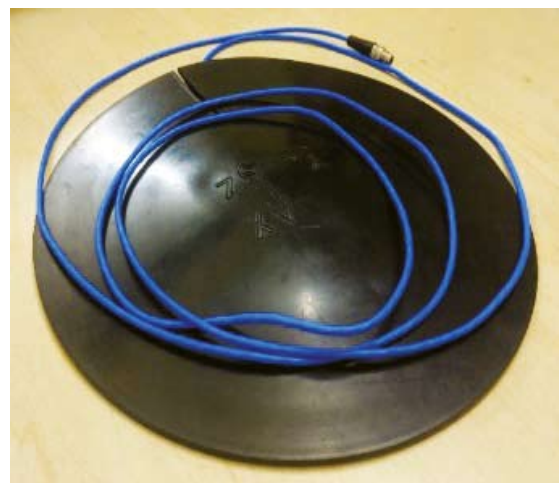
Figure 2. Triaxial Seat Pad Accelerometer
