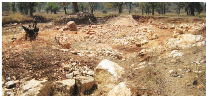
Fig. 2. Completely mined-out pegmatite by surface mining methods. Note remnants of unmined in-situ, elongated quartz core and discarded quartz gravel dumps forming degraded landscape. Locality: Bastar pegmatite belt, Chhattisgarh.
