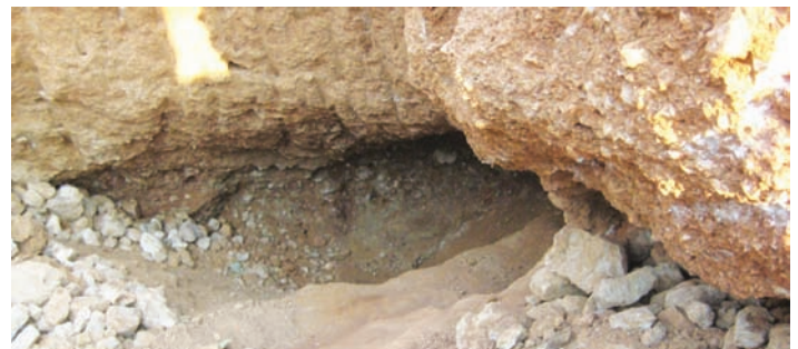
Fig. 3. Small-scale mine (ASM), linear pit in semi-consolidated, pegmatite gravel mining for recovering cassiterite by hand panning. Such underground opening is about 4 metres inside. Locality: Bastar pegmatite belt, Chhattisgarh.
