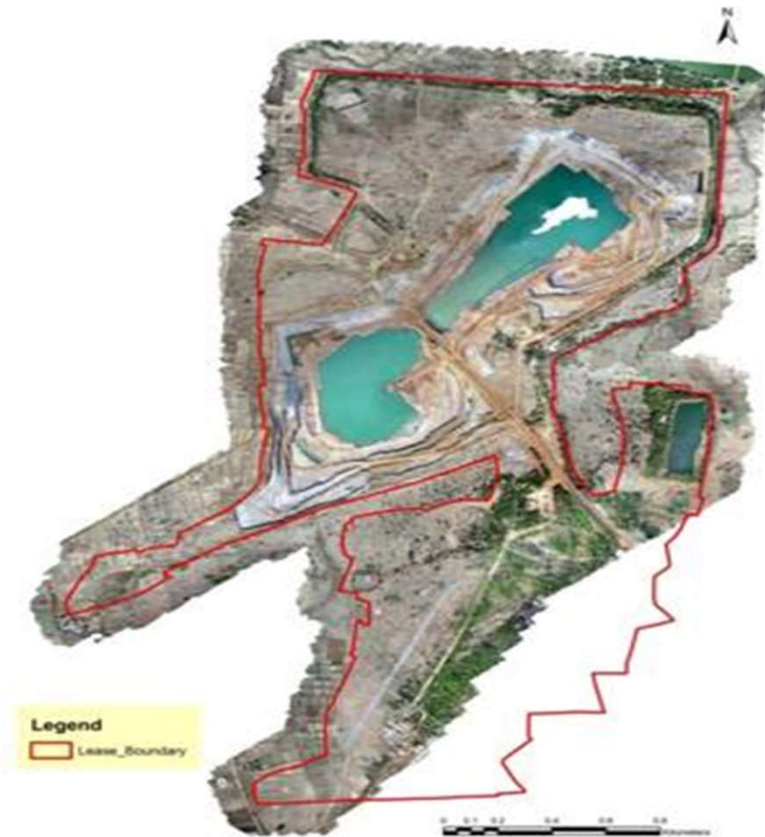
Geo-referenced orthomosaic image generated from UAV Data
