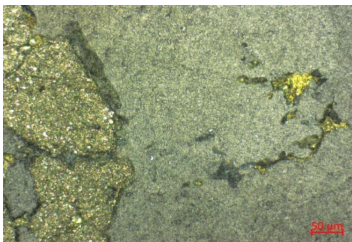
Fig. 3. Microphotograph of blebs and irregular grains of sphalerite and chalcopyrite in quartz
