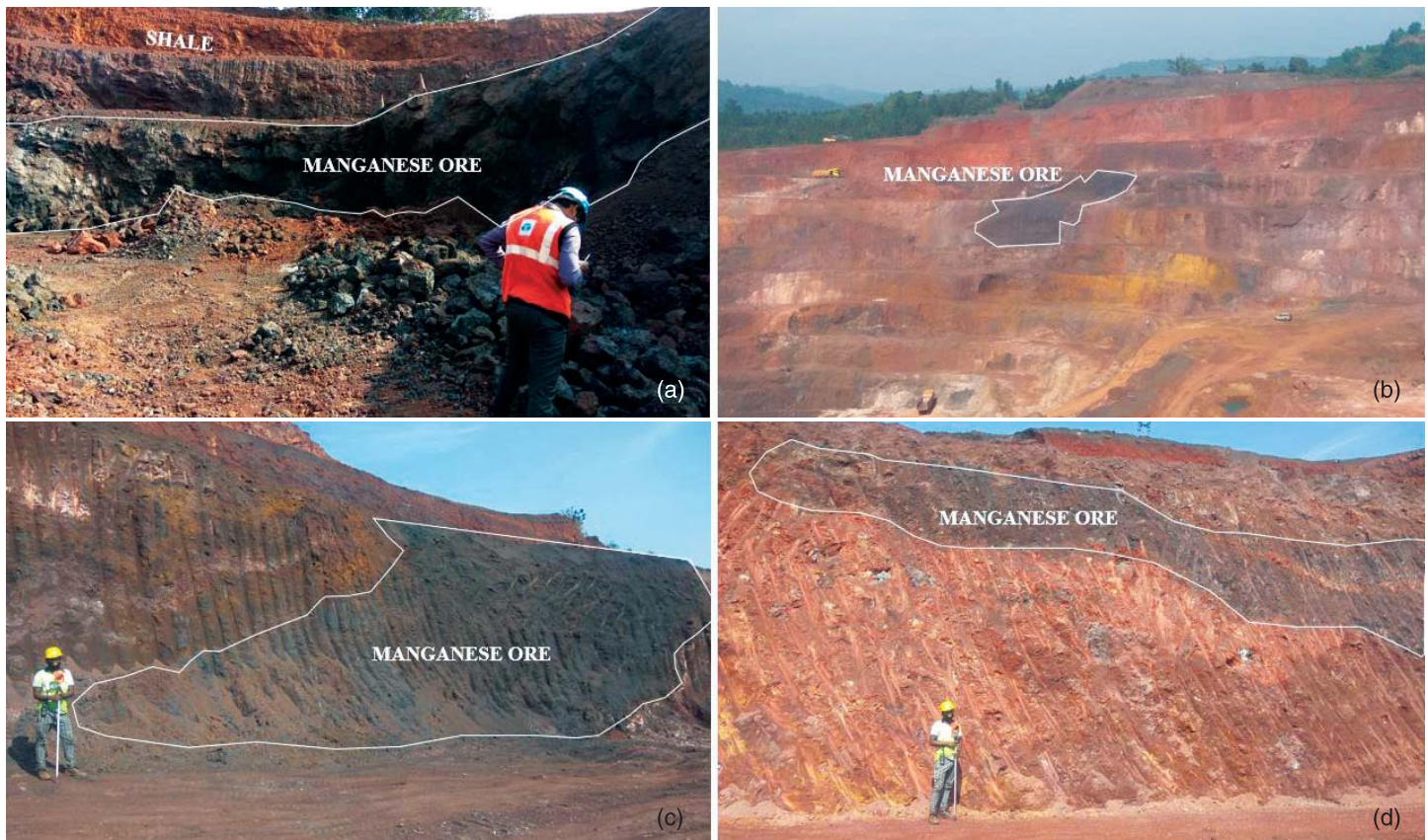
Fig. 2 Field photographs of stratabound type deposit of manganese ore bodies. (a) Stratabound concordant type of deposit at Gurda pit of Tiringpahar. (b) Stratabound discordant type of deposit at Joda west. (c) (d) Stratabound discordant type of deposit at Tiringpahar.
