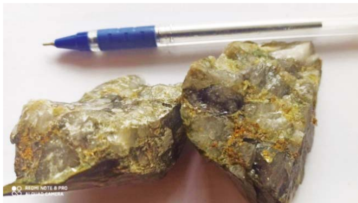
Fig. 2. Sulphide minerals in quartz vein used for wafer preparation for FIS
