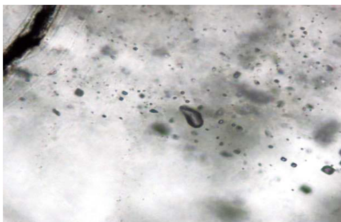
c. Primary monophasic methane inclusions
