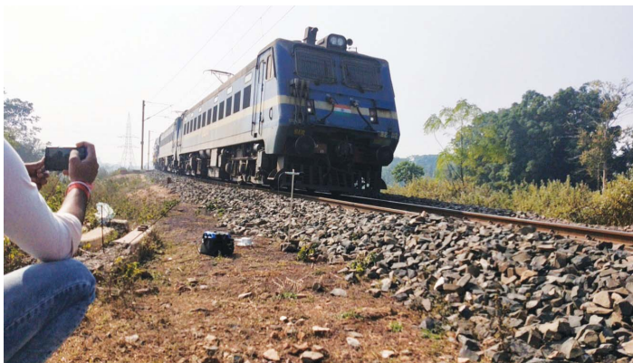
Figure 7. Monitoring of induced ground vibration while movement of train
